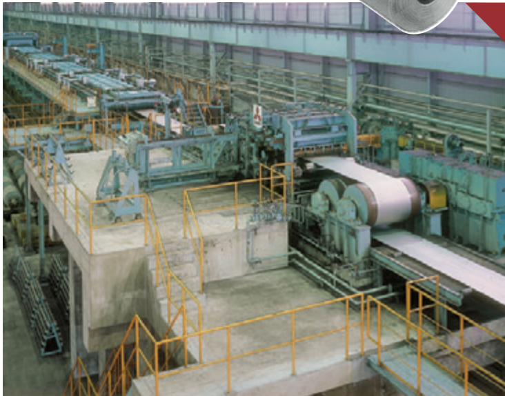
連続酸洗ライン Continuous Pickling Process
