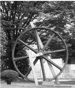
Drawbench main gear from Maruichi Seisakusho era (diameter: approx. 1.8 m)
