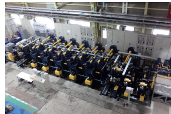
DRW Device (Distortion Correction Unit for Welding Position)
